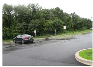
To manage parking lot runoff, parking spaces in the northeastern corner of the parking lot can be converted to pervious pavement. A preliminary soil assessment suggests that the soils have suitable drainage characteristics for green infrastructure.
