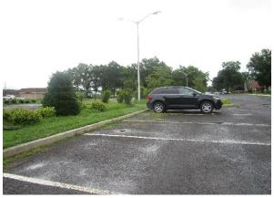
A section of parking spaces on the north side of the parking lot can be replaced with pervious pavement to capture parking lot runoff. A rain garden can be placed in the western section of the island to capture, treat, and infiltrate the parking lot runoff. A preliminary soil assessment suggests that more soil testing would be required before determining the soil's suitability for green infrastructure.
